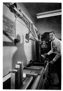
CALIBRATION GAUGE is being used by Stuart A. Ravenbyrne in setting up a radiation micrometer which relates density to thickness.
